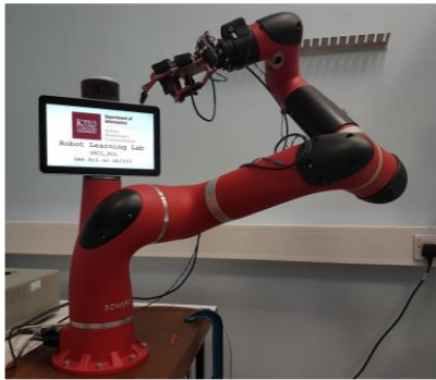
Figure 2: Rethink Robotics Sawyer Robot with AR10 Hand
