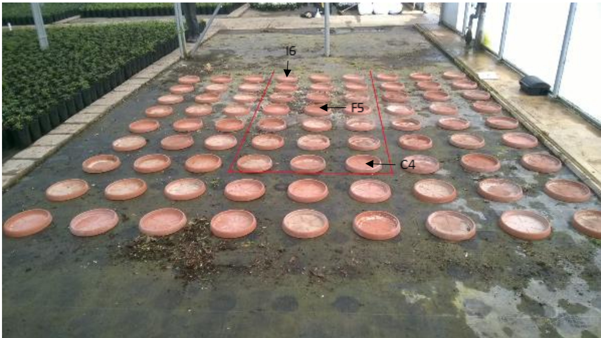
Figure 3.2. Plant pot saucers used to measure water application through the overhead sprinklers in the ‘treatment bay’. Area outlined in red is the selected treatment area. C4, F5, and I6 are three randomly selected pots to assess nematode delivery
