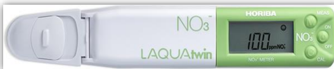
Figure 9. Laquatwin NO 3 sensor used for the nitrate measurement of plant sap
