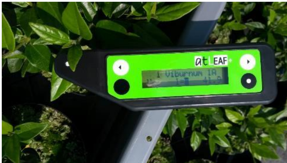
Figure 12. atLEAF+ meter measuring the relative chlorophyll content of green leaf plants.
