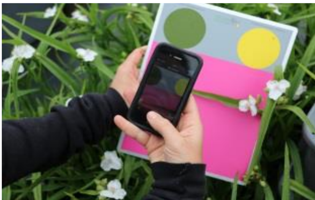
Figure 13. The reference board which acts as a known background to the App used.
