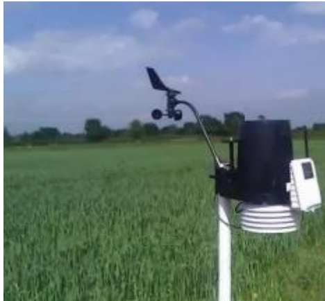
Figures 4 and 5. Wireless Davis Vantage Pro Weather station: in the field (left), and in detail (right).
