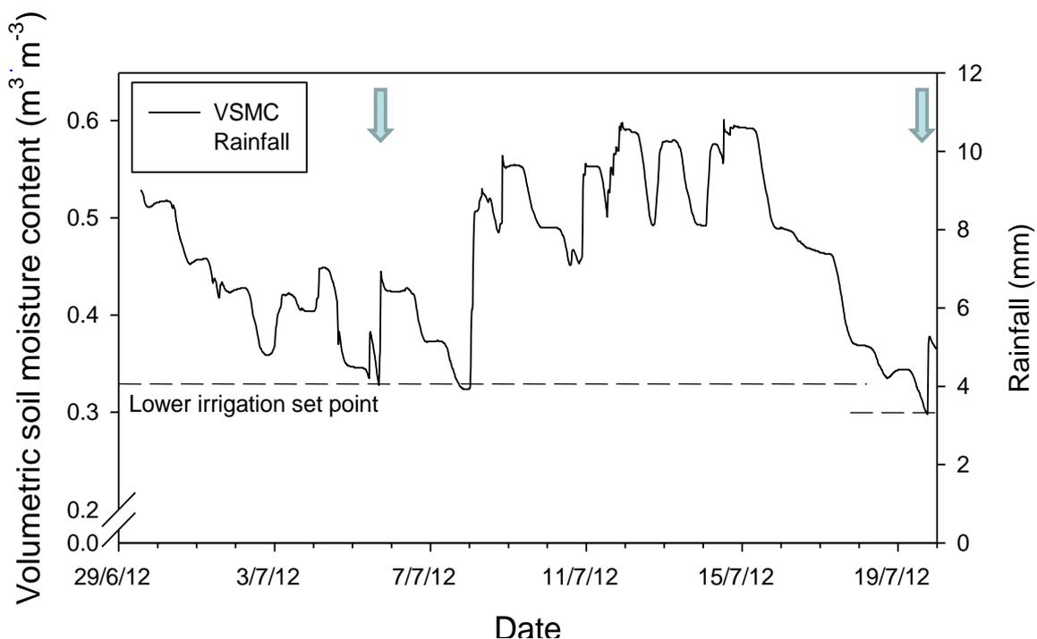
**Figure GS2.** Automated irrigation scheduling prevented over-irrigation of *Escallonia* plants during the wet summer of 2012. Irrigation was triggered automatically on two occasions between 29 June and 19 July 2013 (indicated by the arrows), otherwise, VSMC was maintained above the lower irrigation set points (dashed lines) by frequent and heavy rainfall (blue bars).
