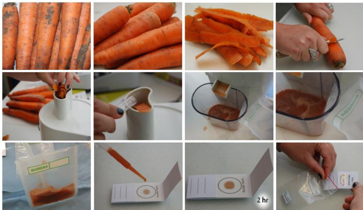
Figure 1. Sampling procedure using the NSure sampling kit. Twenty-five carrots were washed and from each carrot a vertical slice of 10 cm was collected with a potato peeler. The slices were transferred to the juice centrifuge and the extraction fluid was added. The juice was transferred in one half of the extraction bag which contains a sieve. The pipette was used to suck up some juice from the other half of the bag. Two droplets of juice were applied to the sampling card. The cards were dried for at least two hours.
