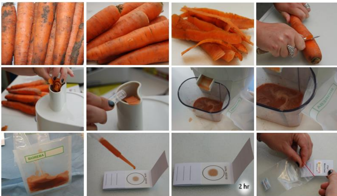
Figure 3. Sampling procedure using the NSure sampling kit. 25 carrots are washed and from each carrot a vertical slice of 10 cm is collected with a potato peeler. The slices are transferred into the juice centrifuge and the extraction fluid is added. The juice is transferred in one half of the extraction bag which contains a sieve. The pipette is used to suck up some juice from the other half of the bag. Two droplets of juice are applied to the sampling card and the cards need to be dried for minimum of 2 hours.
