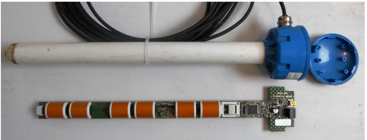
Figure 3 Capacitance soil moisture sensor showing internal construction
