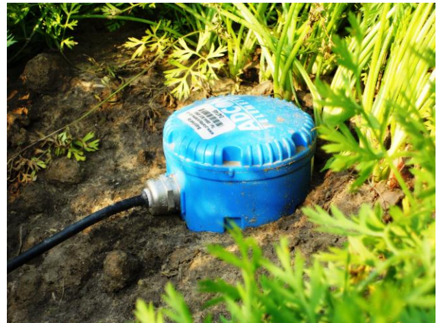
Figure 2 Soil moisture sensor showing insertion into carrot bed alongside row
