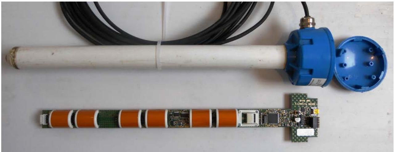
Figure 3 Soil moisture sensor showing internal construction
