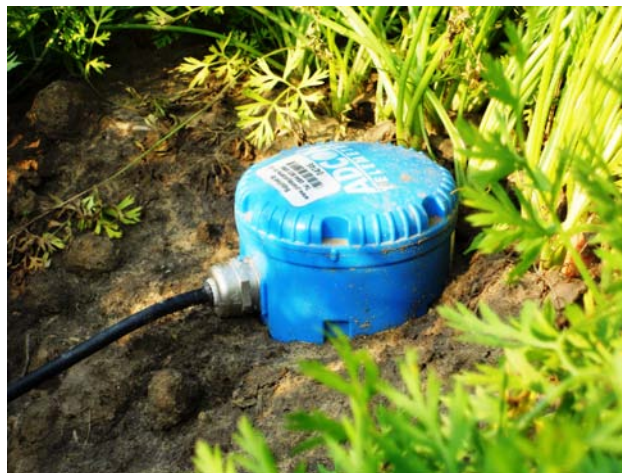
Figure 2: Soil moisture sensor showing insertion into carrot bed alongside rows
