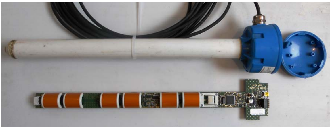
Figure 3: Soil moisture sensor showing internal construction
