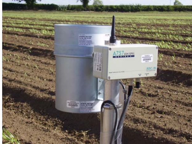
Figure 1: Monitoring station showing RTU and total water input sensor
