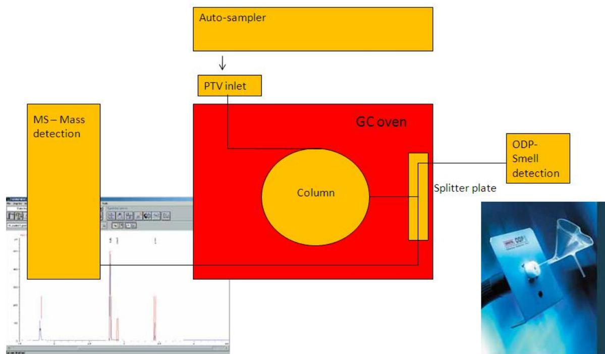
Figure 17. GC-MS/OPD schematic
