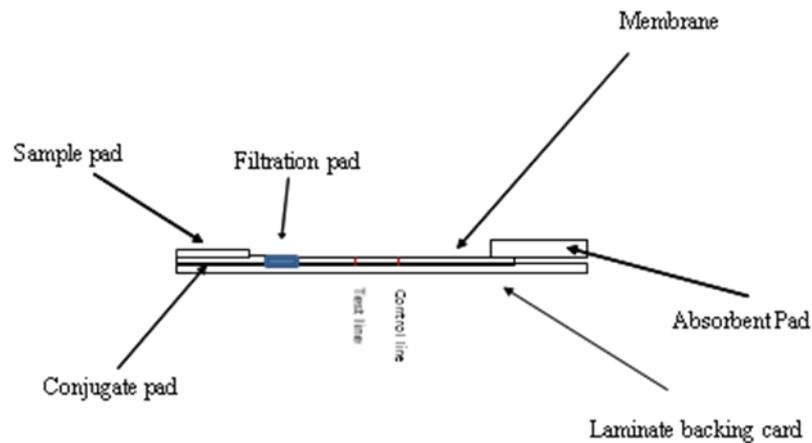
**Figure 12:** Lateral flow device for semi-quantitation of clubroot resting spores
