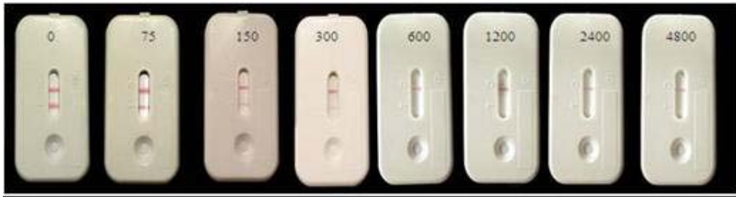
Figure 12 A semi-quantitative competitive lateral flow device with powdery mildew conidial numbers tested between 0 – 4800.
