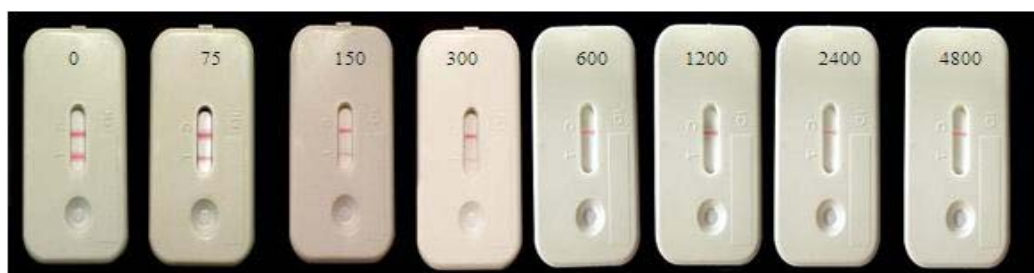
Figure 1 A semi-quantitative competitive lateral flow device with powdery mildew conidial numbers tested between 0 – 4800.
