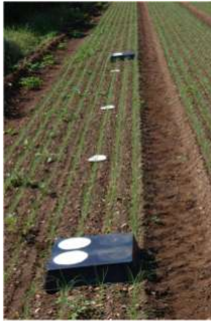
Figure 8. Experimental layout for sampling deposits on horizontal surfaces and onion plants in field conditions
