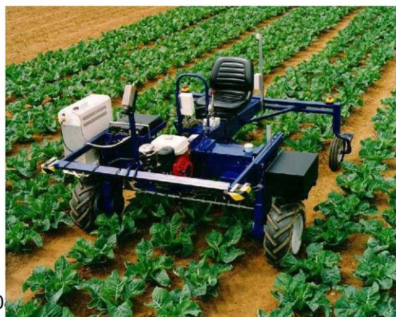
**Figure 23 The toolframe tractor to be used as a platform for the 2008 trial.**
