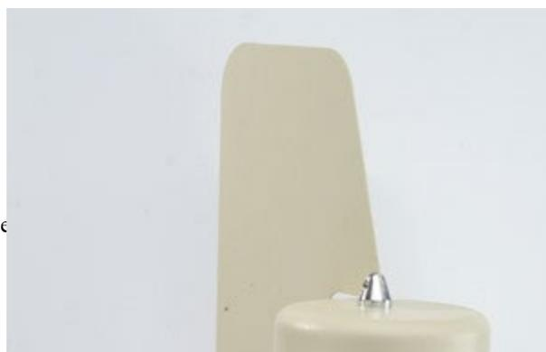
**Fig 2** Portable air sampling device for onion downy mildew conidia
