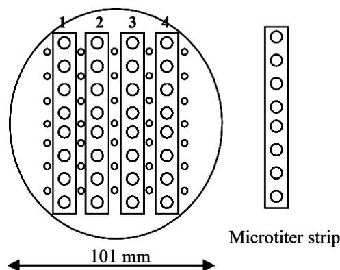
**Figure 9** Schematic drawing of MTIST base plate and microtiter strips.
