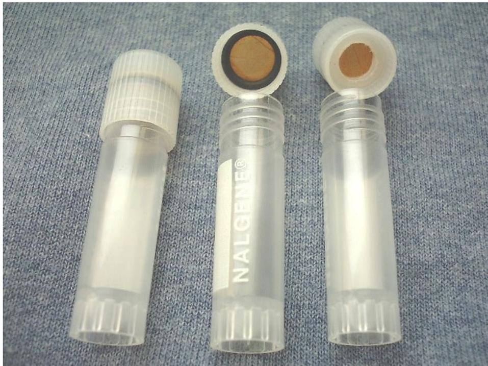
*Appendix Figure 8. Onion skin permeability testing. Tubes for monitoring the passage of water vapour through skin sealed into the cap by measuring loss of weight of the water-filled tube.*
