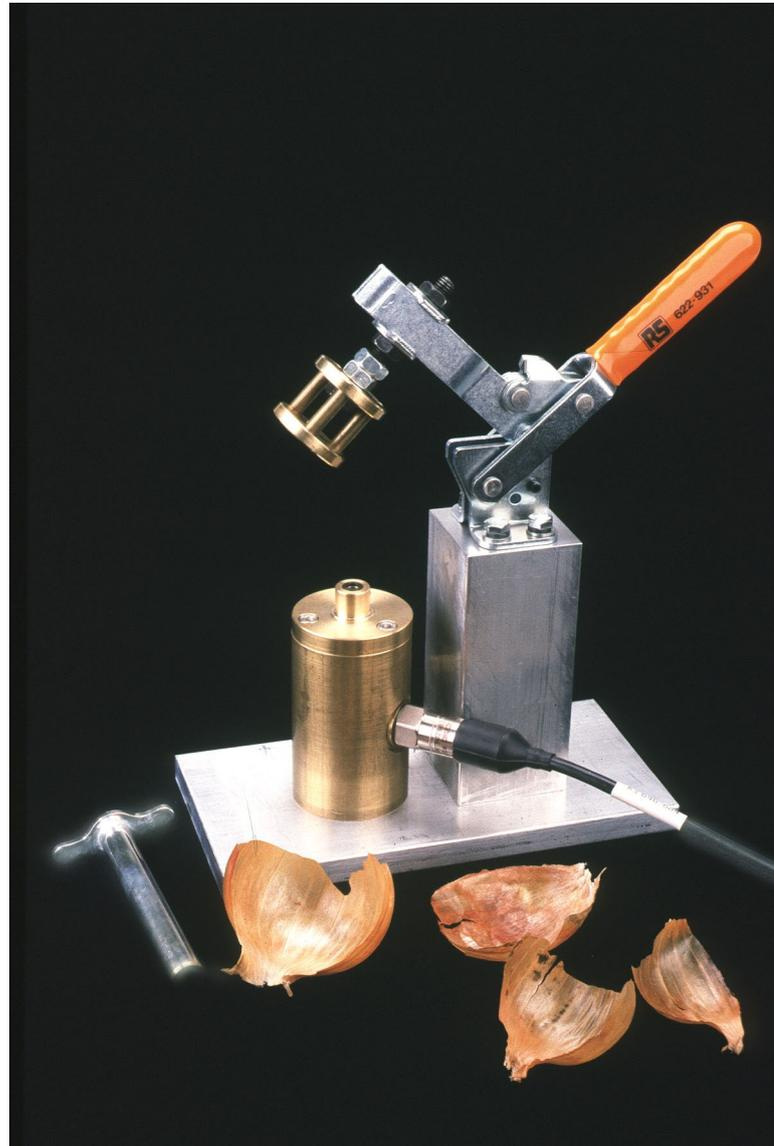
*Appendix Figure 6. Onion skin blaster. Chamber for measuring the pressure at which onion skins fracture when subjected to multi-directional stress from gas pressure.*
