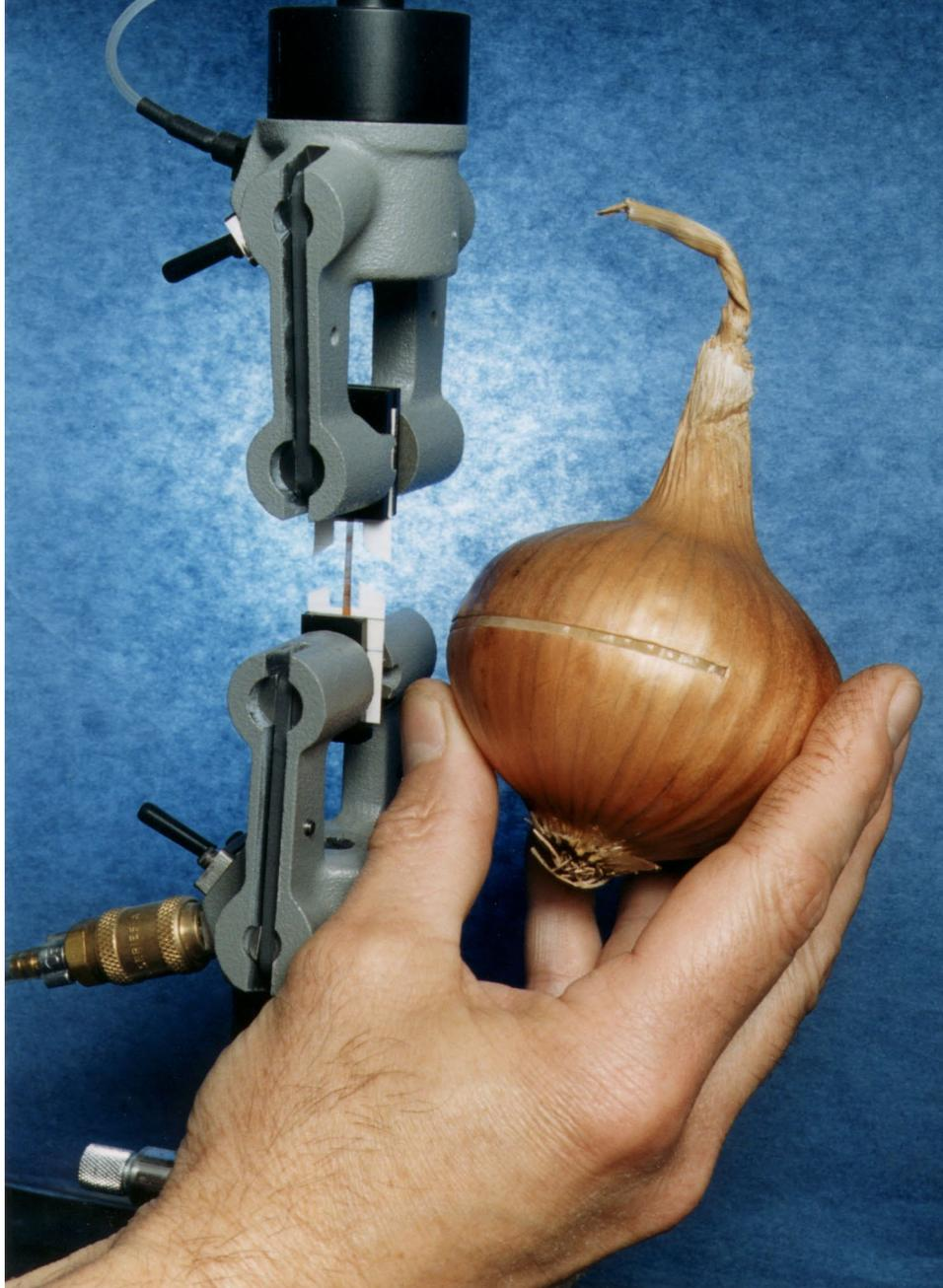
*Appendix Figure 7. Onion skin stiffness. Sample of skin has been removed from bulb and secured into cardboard template before being stretched to failure in grips of materials testing instrument.*
