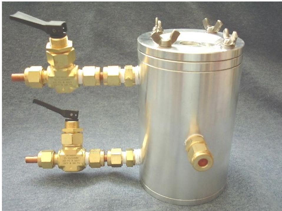
*Appendix Figure 9. Onion skin permeability testing. Chamber for monitoring changes in oxygen and carbon dioxide concentration resulting from passage of gas across skin sealed in to top.*
