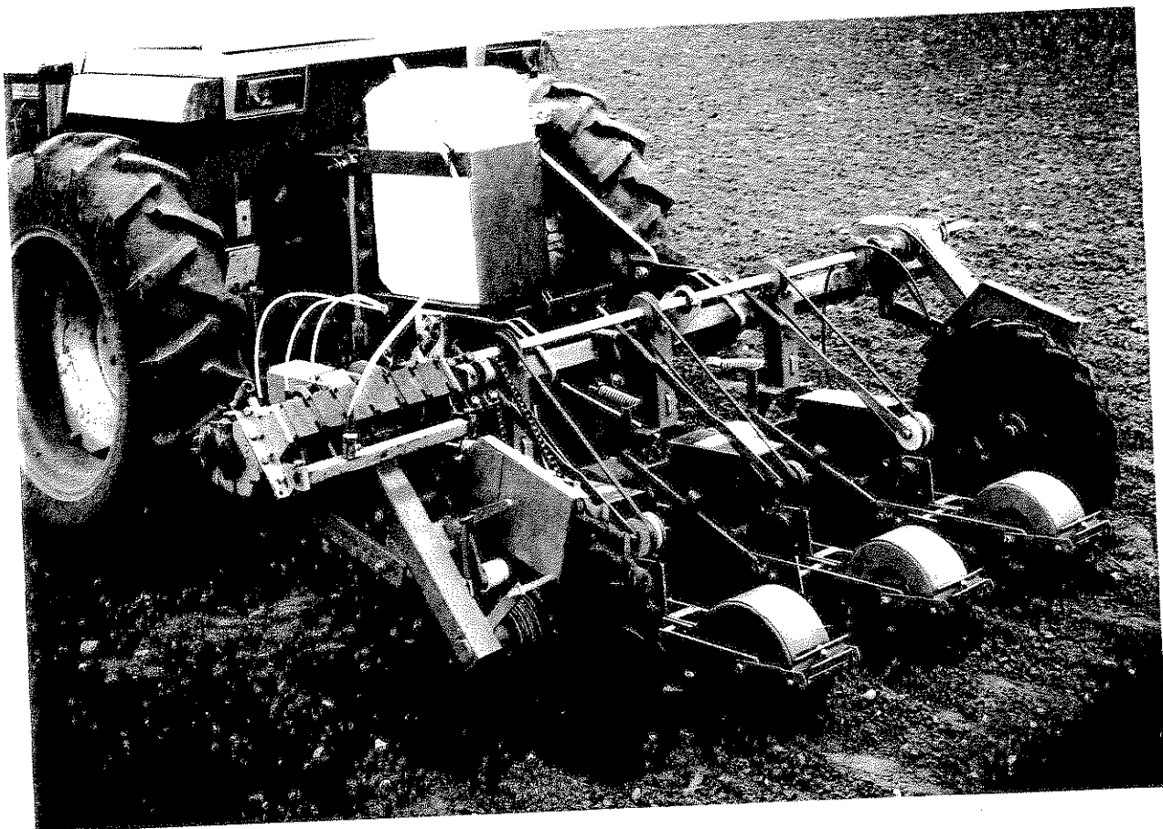
Plate 5. 3-row Stanhay S870 fitted with HRI injection equipment.
