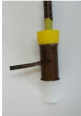
**Figure 6.4** - Metal cylinder with bottle for sap extraction. Photo taken on 18/03/2020.
