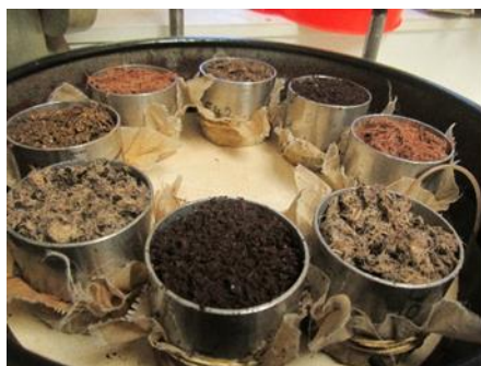
Plate 1. Raw material testing of available water (left) and air filled porosity (right) at ADAS.
