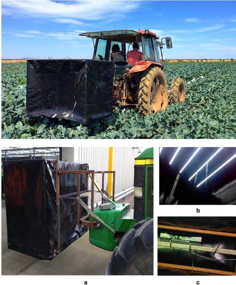
**Figure 3.1:** Data acquisition with the 3D sensor casing mounted at the rear of the tractor is shown in the top picture. In the pictures at the bottom, the sensor (c) is fixed inside a shrouded box (a) to block direct sunlight and to protect the equipment. An arrangement of artificial LED illumination is also fixed inside the box to achieve uniform illumination (b). Images reproduced from [Kusumam et al., 2017], best seen in colour.
