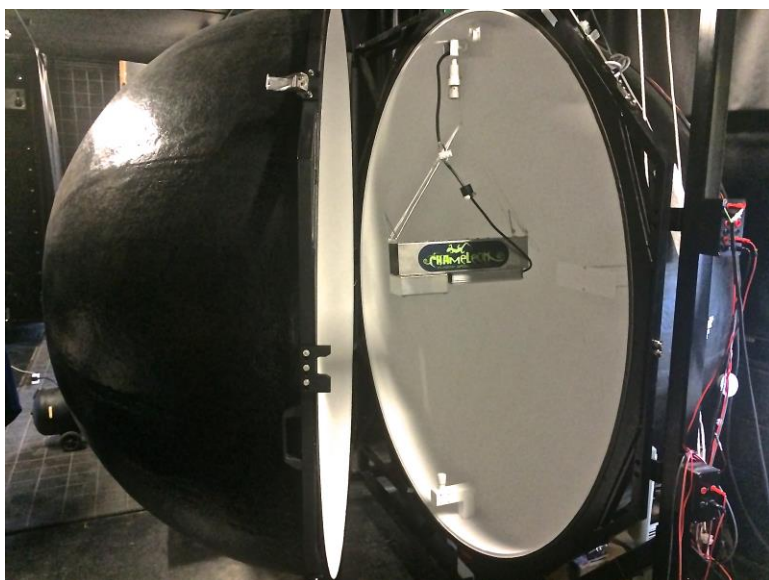
A plasma lamp inside a 1.8m integrating sphere at the LIA laboratory.
