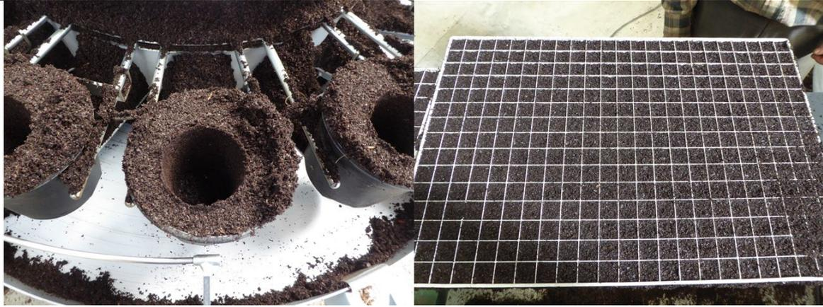
**Figure 79.** Testing prototype blends on a pot filling machine (2 L pots) and a tray-filling machine (345-cell trays).
