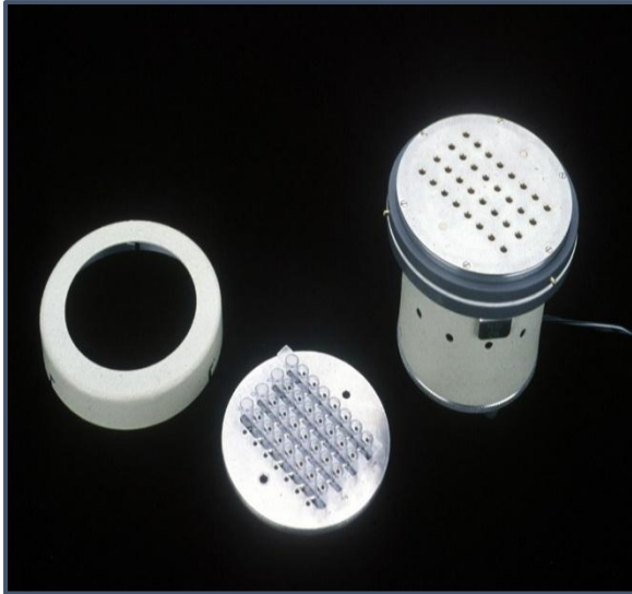
Figure 1. MTIST air sampler with base plate containing 4x8 well microtitre strips.
