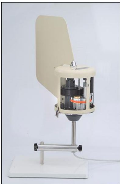
Figure 1c. Multi-vial air sampler with eight collection tubes.
