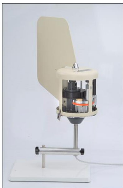
Figure 1c. Multi-vial air sampler with eight collection tubes.
