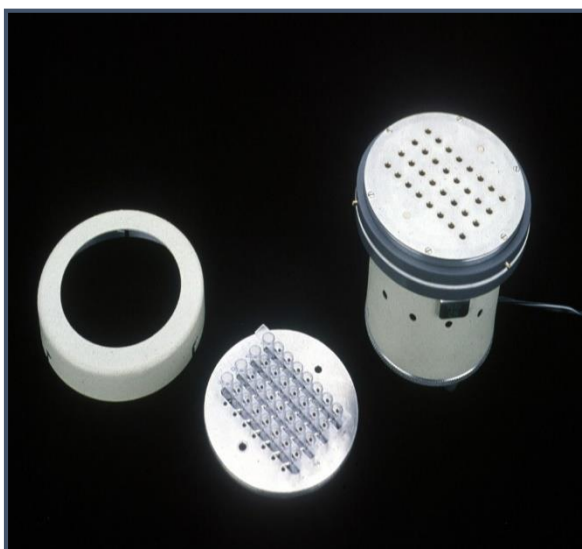
Figure 1a. MTIST air sampler with base plate containing 4x8 well microtitre strips.
