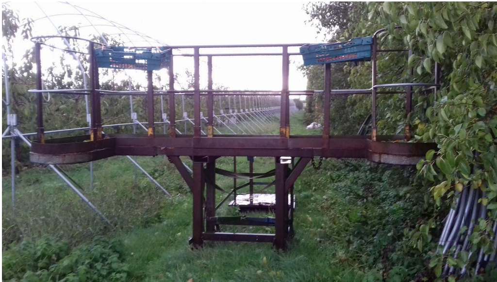
Figure 1. In-house polytunnel forklift rig to aid tunnel ‘skinning’
