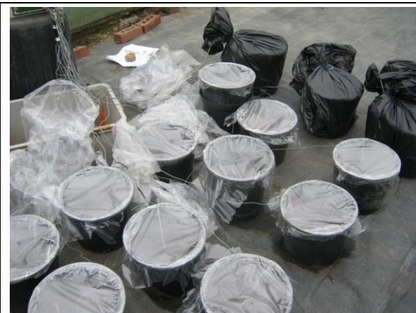
Figure 3. Pots in randomised block with first plastic cover and some already sealed in black plastic bags to further ensure a seal
