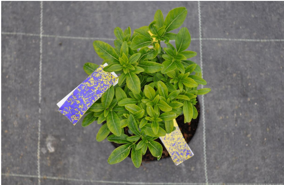
Figure 1. Spray coverage on water-sensitive paper at 750 L/ha
