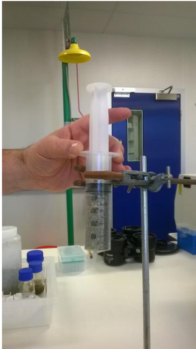
Figure 18. A disposable 50ml syringe packed with a china clay sand mix prior to soil filtration (soil size exclusion)
