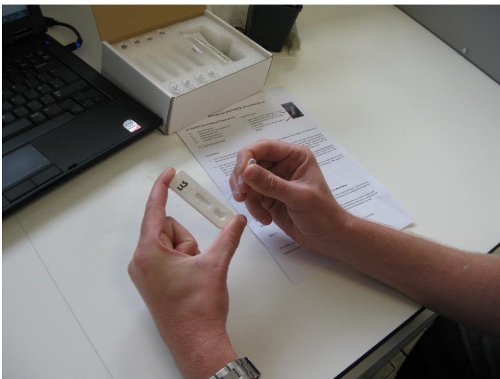
Figure 7. Grower diagnostic kit: Transfer of the field bioaerosol sample to the light leaf spot lateral flow test
