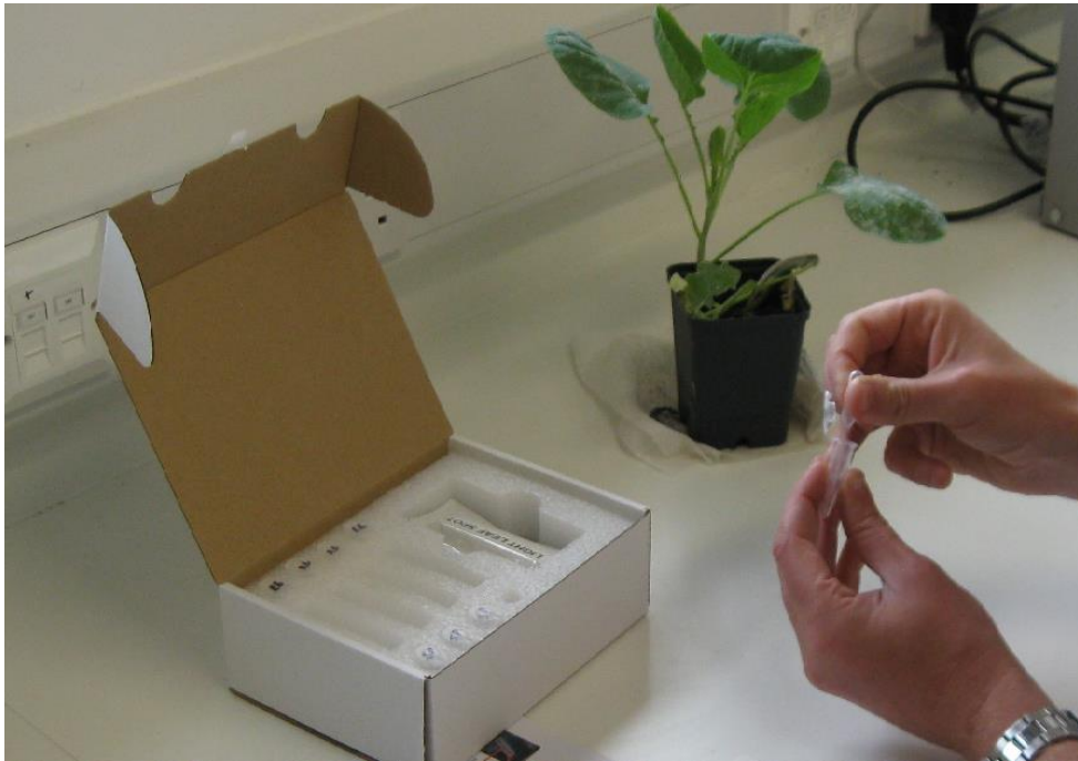
Figure 6. Grower 'in field' light leaf spot diagnostic kit: Application of buffer (NPARU B2) to the field bioaerosol sample.
