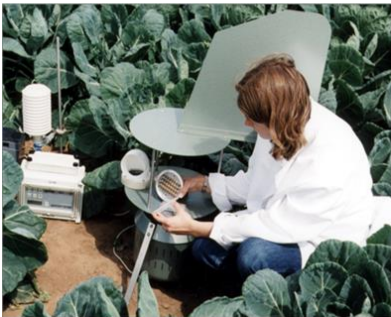
Figure 4. MTIST air sampler positioned within a commercial Brussels sprout cropping system and operated from an environmental data logger
