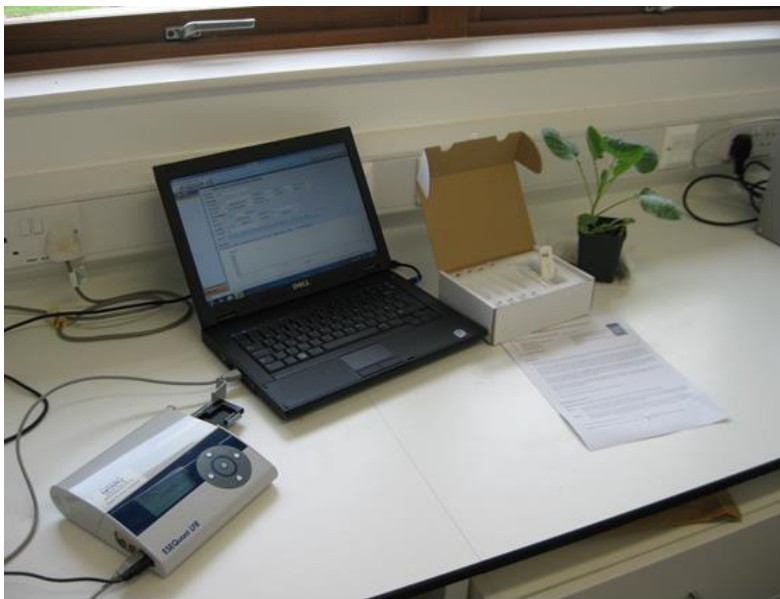
Figure 8. Quantitative measurement (electronic record) of the test using a portable ESE lateral flow reader.
