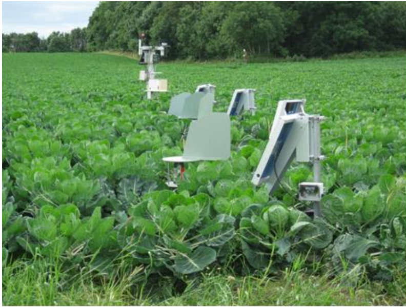
Figure 3. Environmental data logger and four field bioaerosol (air) samplers sited in a Brussels sprout crop in the East of Scotland
