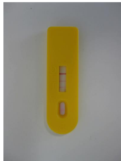
Figure 13. Multiplex lateral flow device for the measurement of Albugo candida (white blister) and Erysiphe cruciferarum (Brassica powdery mildew): two test lines for independent measurement of each spore type and a control line.
