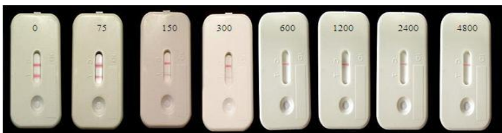
Figure 1. A competitive lateral flow assay with powdery mildew spore numbers measured between 0 – 4800.
