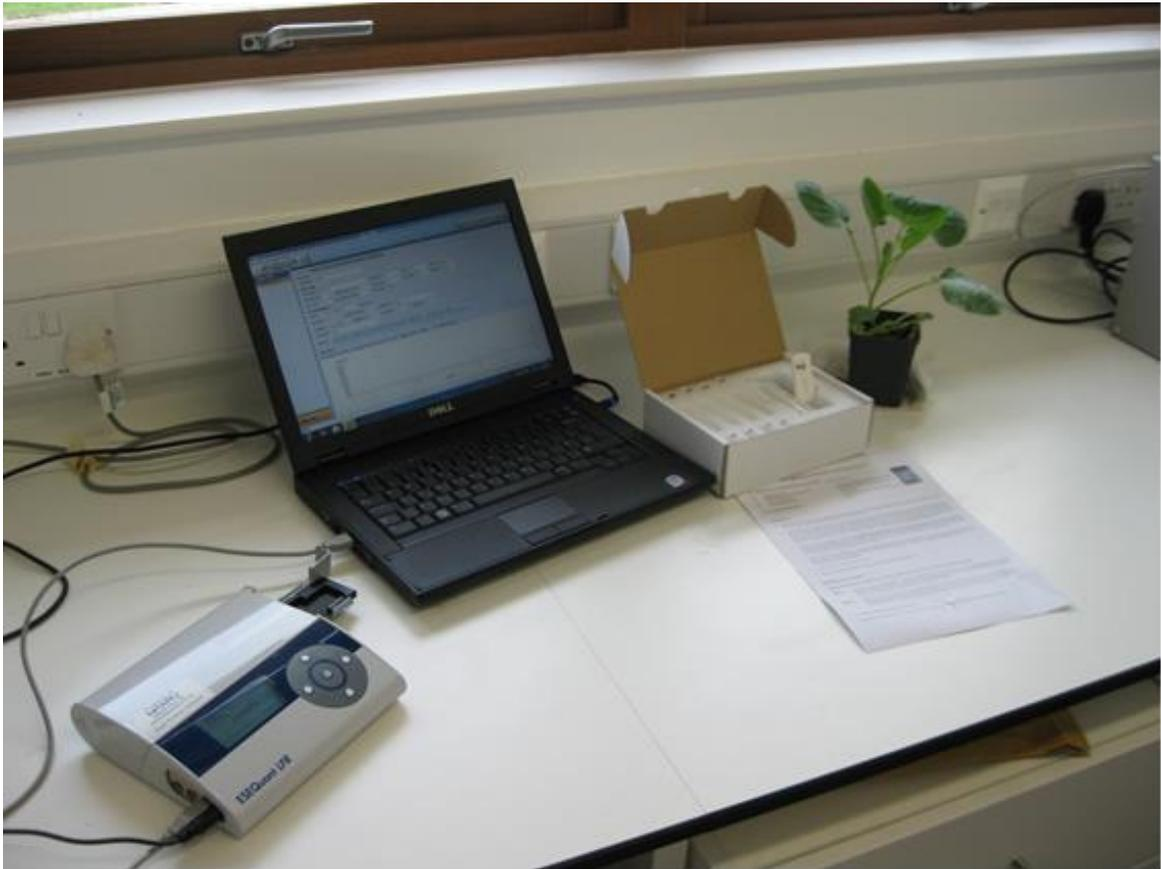
**Figure 8.** Quantitative measurement (electronic record) of the test using a portable ESE lateral flow reader.
