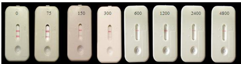
Figure 1. A semi-quantitative competitive lateral flow assay with powdery mildew conidial numbers tested between 0 – 4800.
