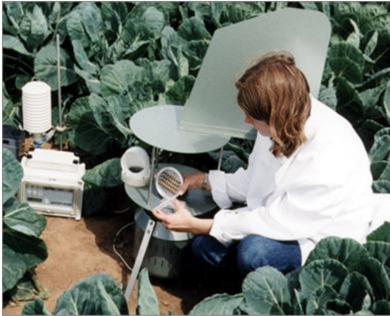
Figure 5. MTIST air sampler positioned within a commercial Brussels sprout cropping system and operated from an environmental data logger
