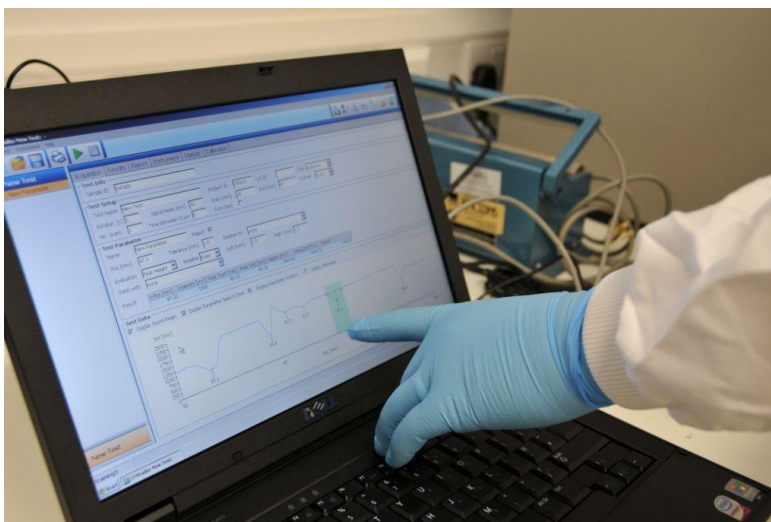
Figure 4b. Lateral flow test and control line digital output as displayed on a portable lap top screen
