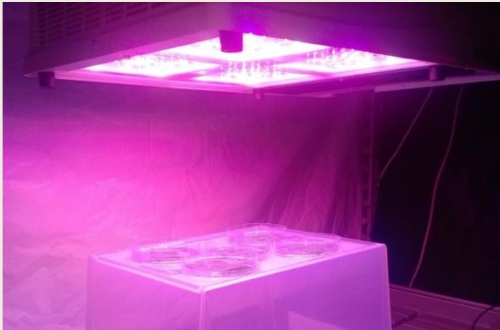
Figure 2. Experimental setup showing leaves in petri dishes located directly under one of the Heliospectra lamps.
