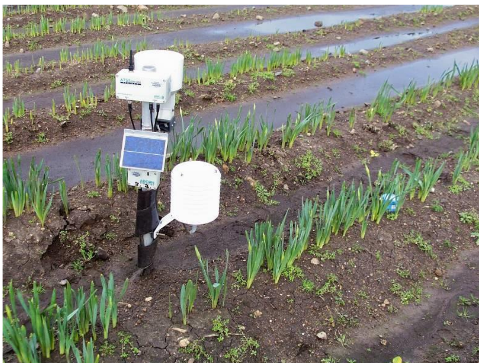
Figure 3. One of Plantsystems ‘Active Irrigation Scheduling’ monitoring station on site
