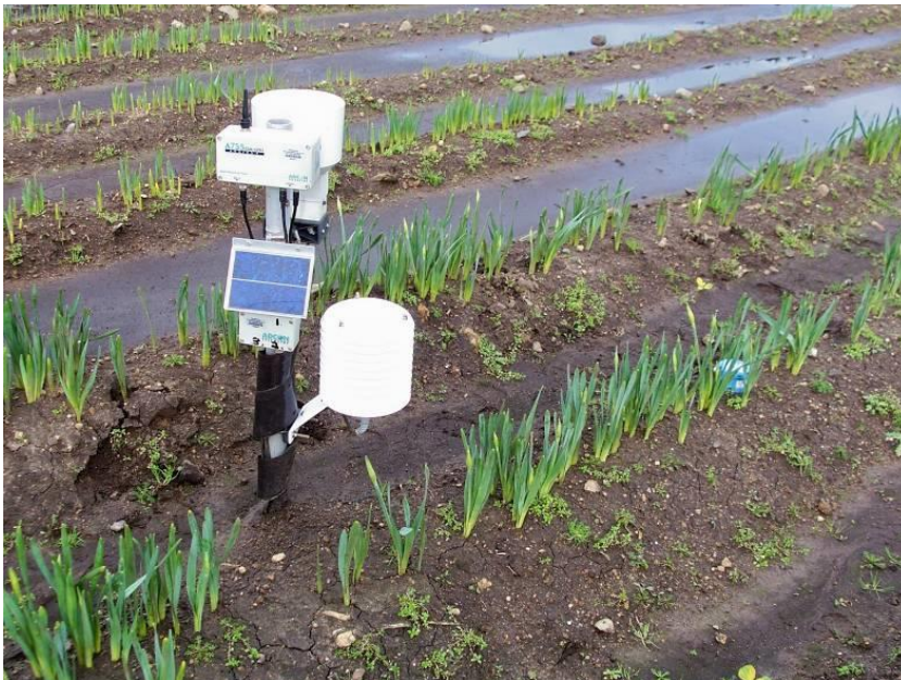
Figure 3. Plantsystems (Agrovista) 'Active Irrigation Scheduling' monitoring station on site.
