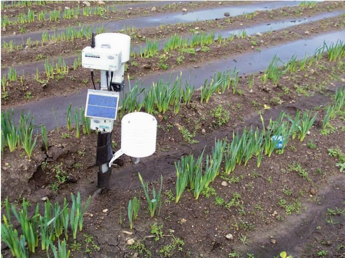
Figure 8. Plantsystems (Agrovista) 'Active Irrigation Scheduling' monitoring station on site.
