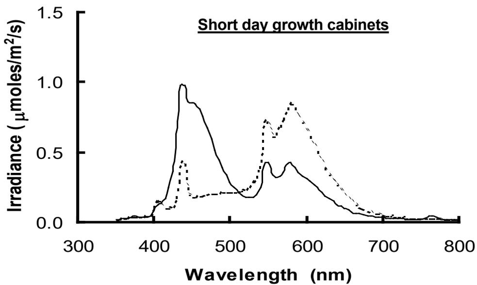
**Figure 1.1.** Light quality of the four growth cabinets used to assess the effects of photoperiod and blue light enhancement on shoot/bulb formation by snowdrop bulb chip explants. Cabinets were fitted with either cool white fluorescent tubes (dashed line) or mixture of cool white fluorescent tubes and Osram L 36W/67 blue fluorescent tubes (solid line).
