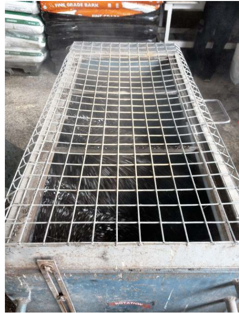
Figure 2. Mixer used for mixing propagation mix for plugs and herbaceous mix for potting up
