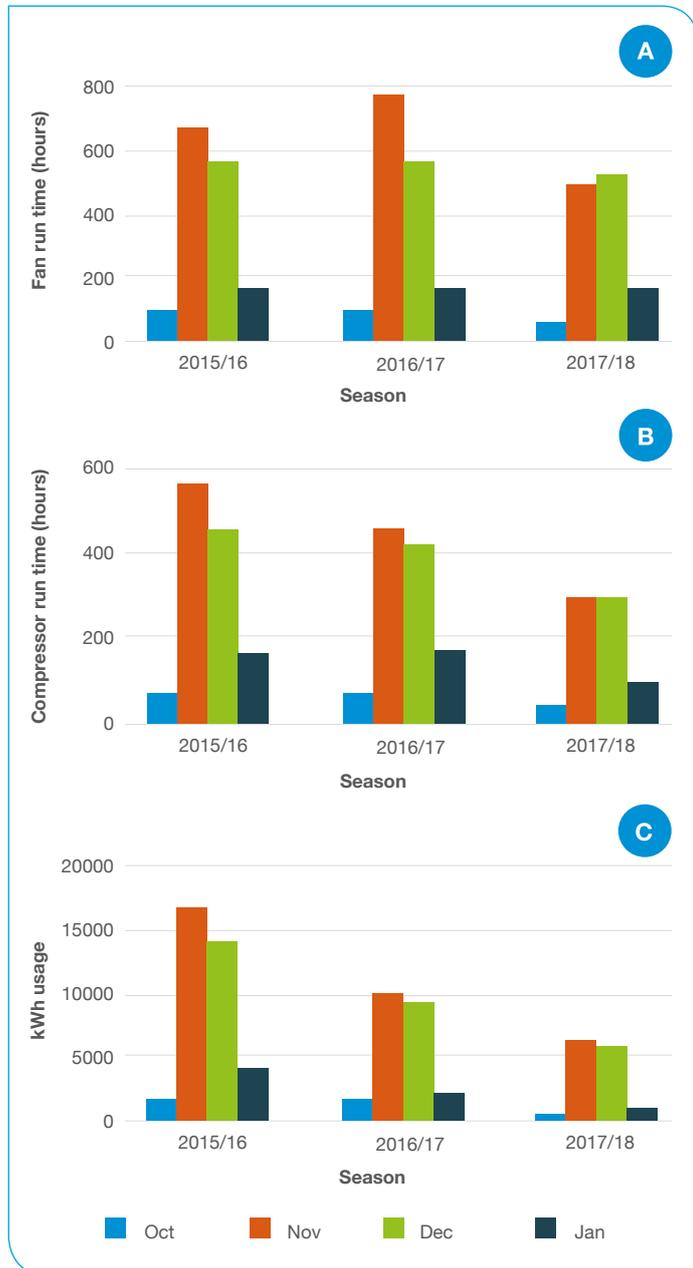
Figure 2. Monitoring of plant running times and energy costs following improvements. A. Fan run times, B. Compressor run times, C. Energy (kWh) savings over time
