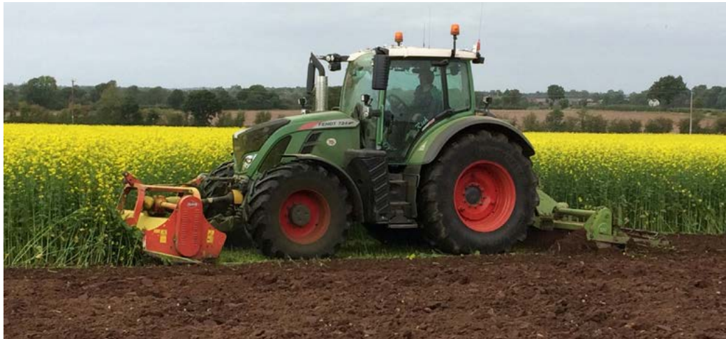
Figure 1. Maceration and incorporation of a mid-flowering Indian mustard biofumigant crop using a flail-topper (A) and rotavator (B)
