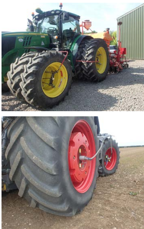
Figure 8. Retro-fit central tyre inflation system (CTIS) options (left, top and bottom) and original-fit, fully integrated CTIS (right)
