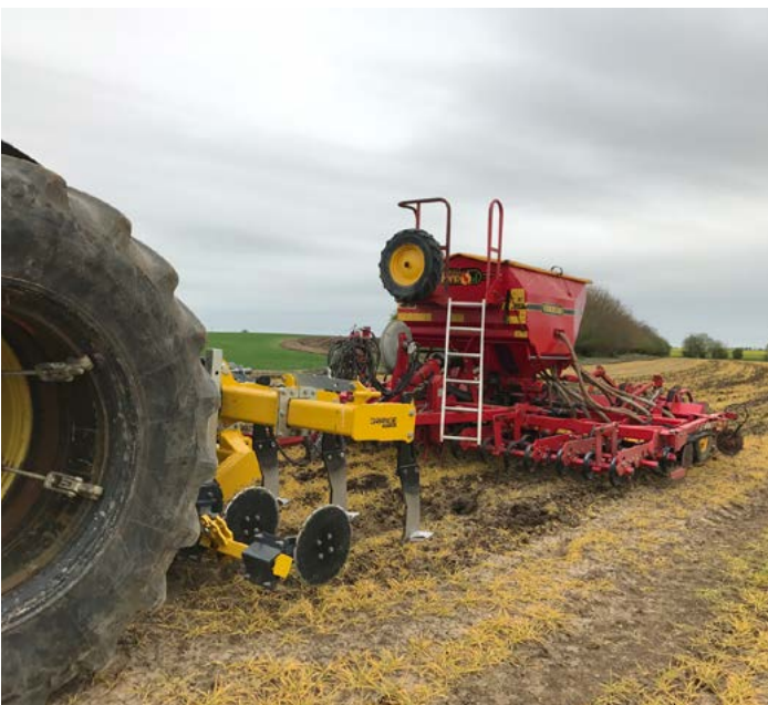
Figure 31. Combined structuring and drilling (left) and cultivator drill used as a direct drill with cultivation elements raised clear of work (right)
