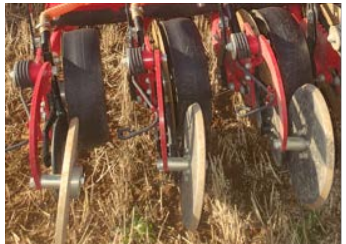
Figure 34. Angled disc opener (left) and straight disc openers with side gauge wheels (right)
