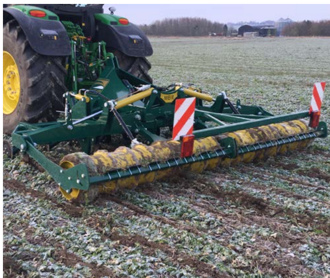
Figure 13. Soil loosening through a growing cover crop
