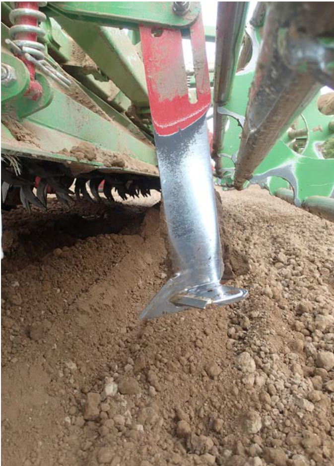
Figure 40. Option to loosen below the pick tines of a bed-former, aligned to the rows that will be planted next
