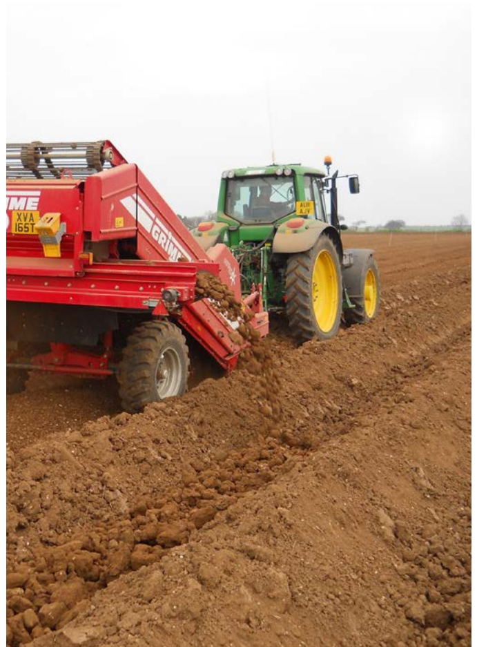
Figure 41. When destoning, monitor depth for improved work rates and fuel consumption
