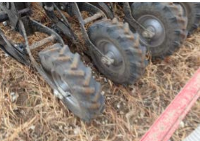
Figure 34. Angled disc opener (left) and straight disc openers with side gauge wheels (right)
