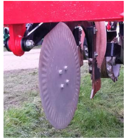
Figure 32. Examples of tine-based drills with leading discs. These enable effective operation in higher levels of residues and reduce soil disturbance
