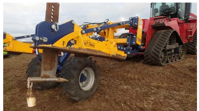
Figure 1. Mole drains are formed by dragging a 'bullet' followed by an expander through the soil to form a circular semi-permanent channel
