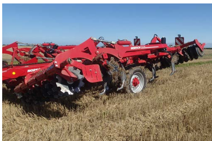
Figure 24. Lower surface disturbance, shallower discing machine option
