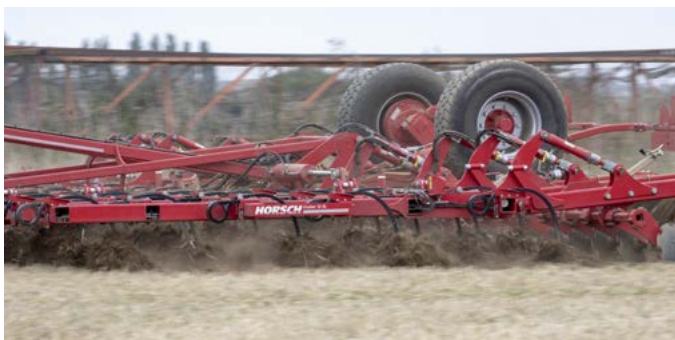
Figure 27. Shallow tine-type cultivator with multiple rows of narrow-tipped tines
