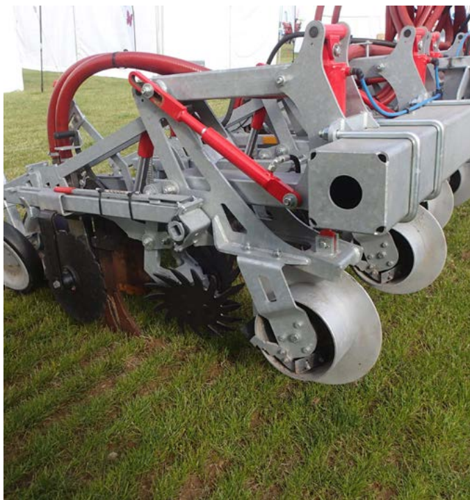
Figure 30. Example of leading and side-border discs, with leading residue manager wheels
