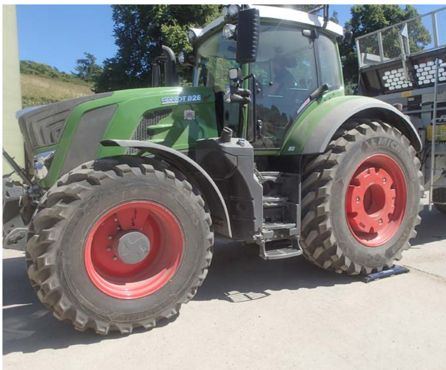
Figure 8. Retro-fit central tyre inflation system (CTIS) options (left, top and bottom) and original-fit, fully integrated CTIS (right)
