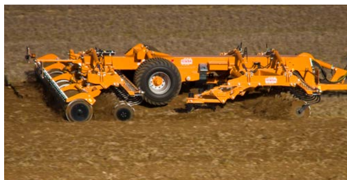
Figure 23. Typical high disturbance, deep non-inversion mixing action
