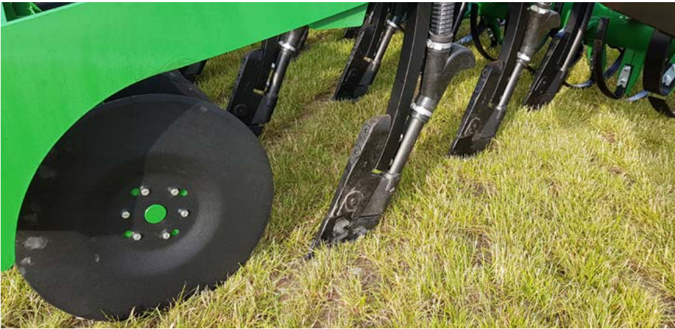
Figure 32. Examples of tine-based drills with leading discs. These enable effective operation in higher levels of residues and reduce soil disturbance
