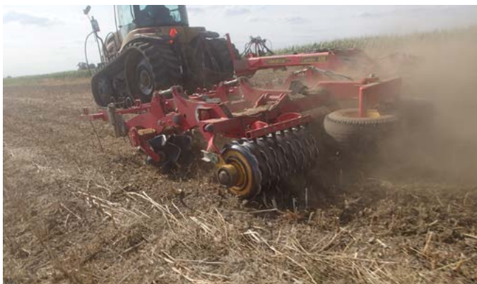
Figure 26. Wave-type discs on a shallow non-inversion cultivator
