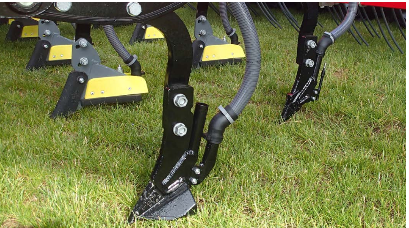
Figure 33. Alternative openers for a tine drill to modify the amount and degree of soil disturbance and drilling band width
