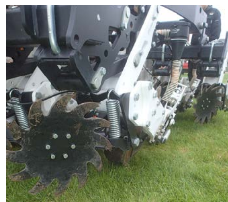
Figure 5. Example of residue managers fitted ahead of drill coulters
