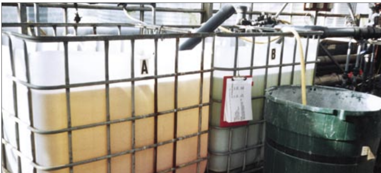
7 To avoid insoluble precipitates and blockage in the irrigation system, calcium should always be added separately from phosphates or sulphates
