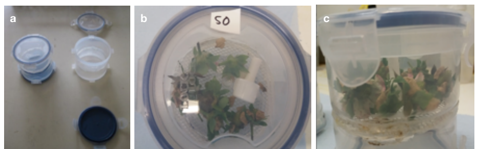
Figure 1. Extraction devices when empty (a) and containing 10 button fruit when set up for experiment (b) overhead view with the MIK dispenser visible, (c) side view
