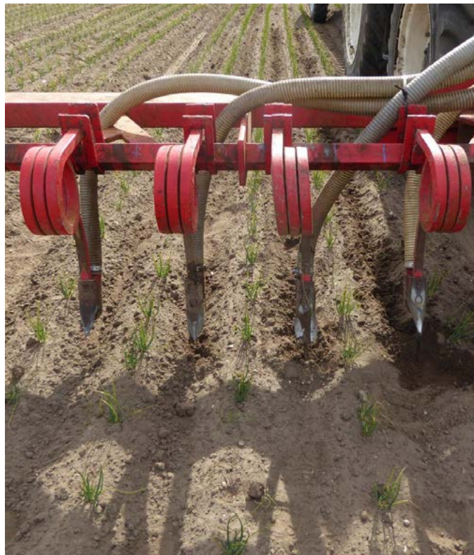
Slurry injection system
