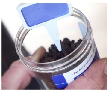
Figure 2. The Solvita® soil health test measures the carbon dioxide evolved from respiration of soil organisms
