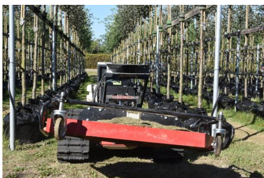
Aebi mulcher, controlled by Robot Makers, being used on standard trees.
