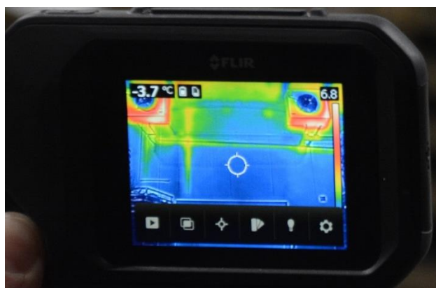
View of the cold store door, with two evaporators above it with a normal and an infra-red heat imaging camera.
