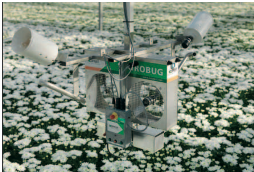
15 The 'Airbug' automatic applicator from Koppert
