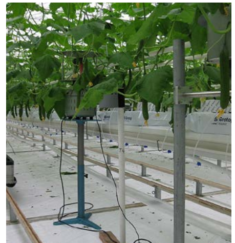
Figure 2. Burkand air sampler collecting spores in a cucumber crop
