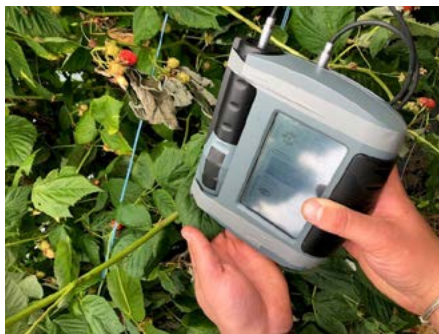
Figure 1. A hand held imaging device and fluorescent tracer were used to access spray deposition
