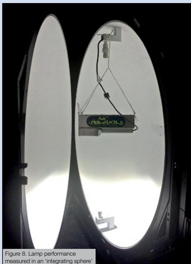
Figure 8. Lamp performance measured in an 'integrating sphere'
