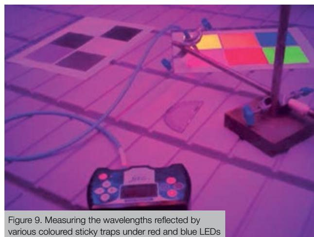
Figure 9. Measuring the wavelengths reflected by various coloured sticky traps under red and blue LEDs
