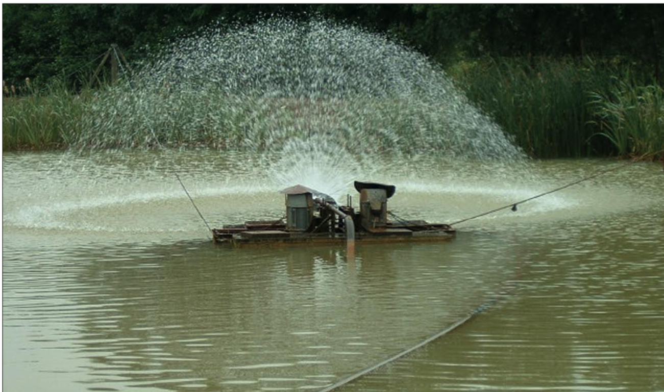
17 Various forms of aeration can be employed to provide some control of algae
